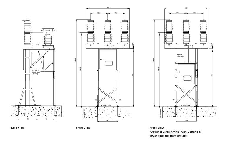
Standard feature is of Fixed height structure. Optional version of telescopic structure to vary mounting height and CT or PT mounting arrangement can be provided on request.
